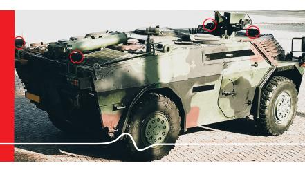
THE MSRA FIRMWARE, BASED UPON A DISTRIBUTED MESH NETWORKED ARRAY OF PASSIVE VEHICLE MOUNTED CASTLE SENSOR POSTS, IS DESIGNED FOR COUNTER BATTERY PURPOSES.
